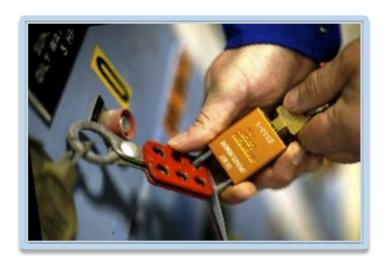
The basic steps of performing lockout/tagout procedure are as follows:
