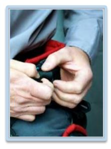
You must look for any visual signs of any significant defect: such as tears, cuts, abrasions, undue stretching, mold, or anything that might cause the system to fail.
